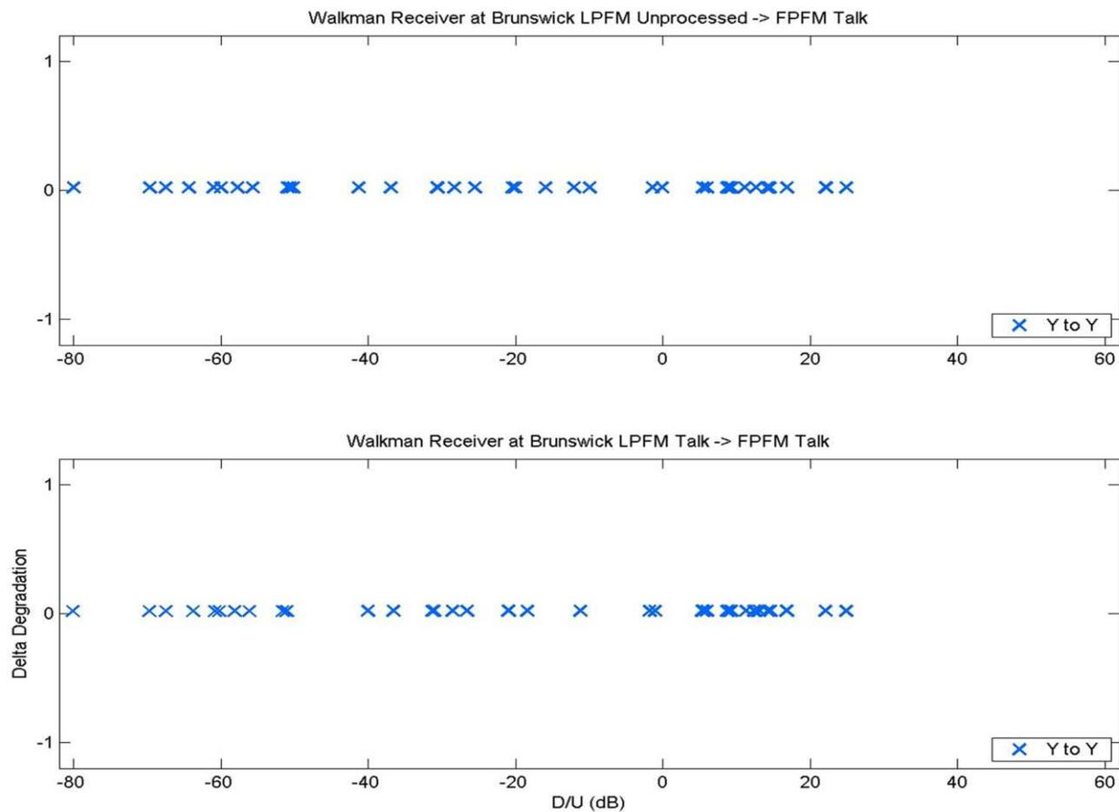
**Figure E-9. Delta Degradation for the Walkman Receiver at Brunswick and for the Specified LPFM-FPFM Program Content Combinations**
