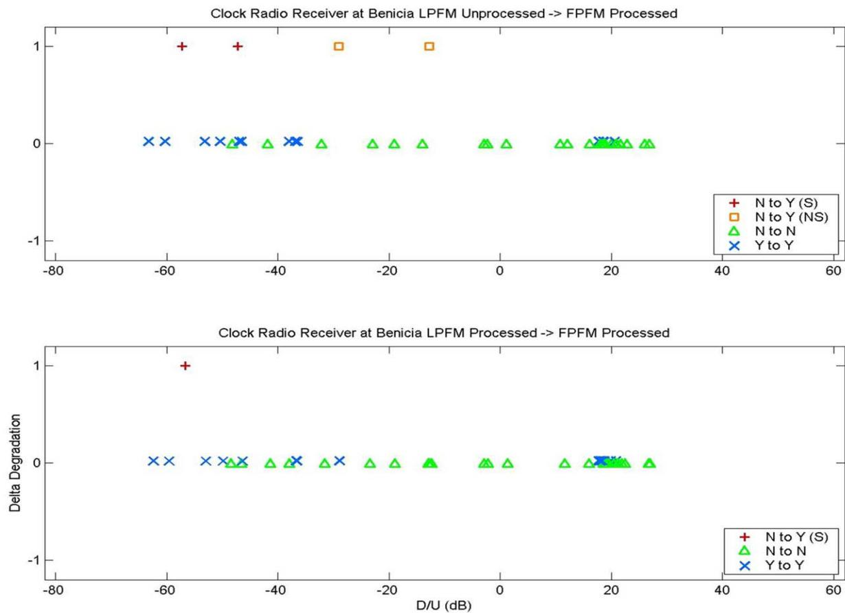
**Figure E-28. Delta Degradation for the Clock Radio Receiver at Benicia and for the Specified LPFM-FPFM Program Content Combinations**
