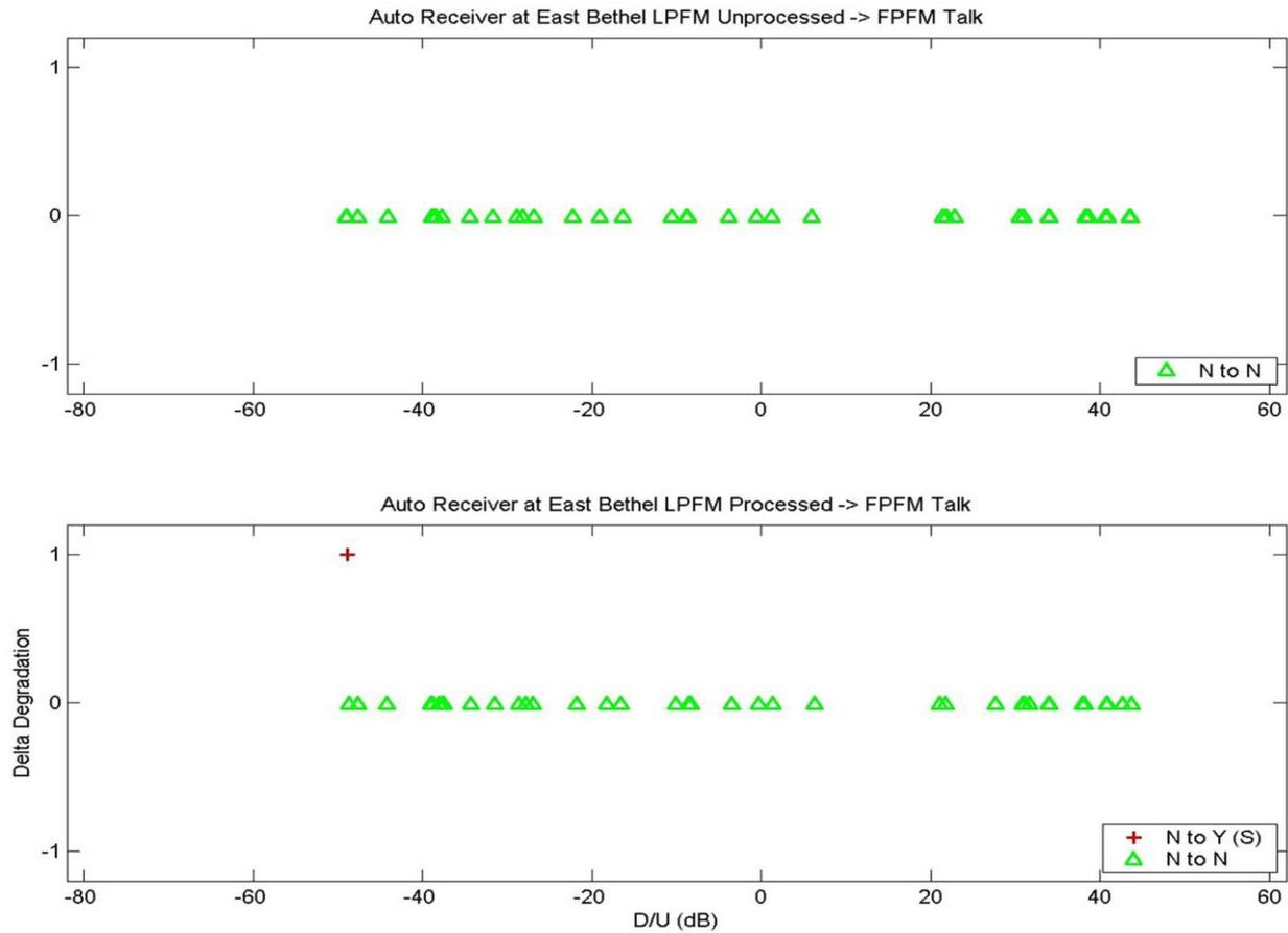
**Figure E-11. Delta Degradation for the Auto Receiver at East Bethel and for the Specified LPFM-FPFM Program Content Combinations**
