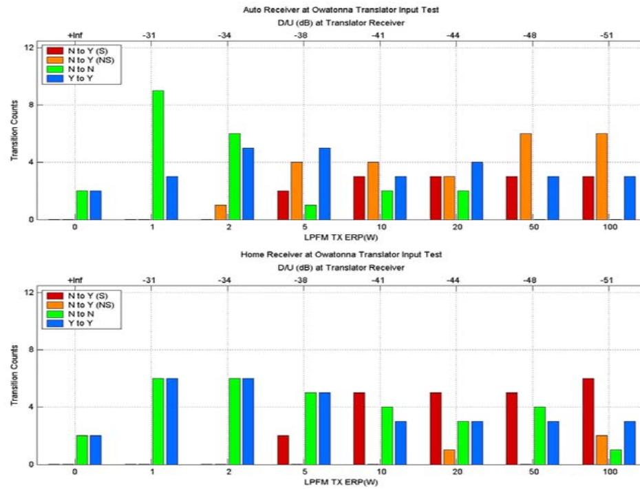
**Figure C-13. Transition Counts for the Auto and Home Receivers at Owatonna Translator Input Test**
