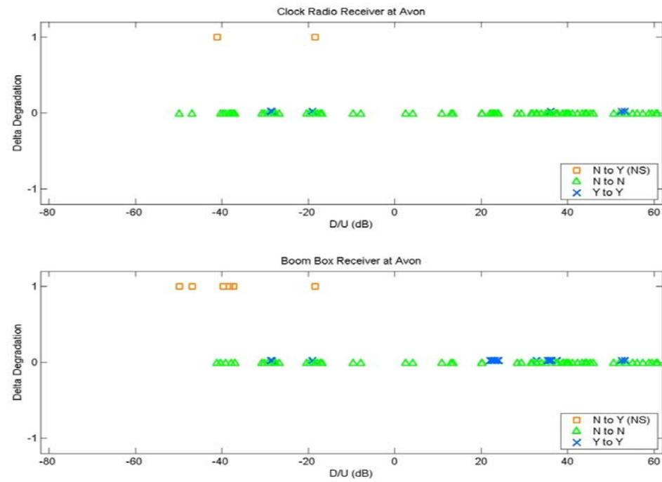
**Figure C-2. Delta Degradation for the Clock Radio and Boom Box Receivers at Avon**
