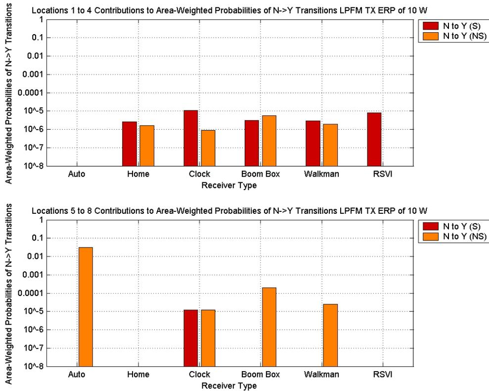
**Figure 2-7. Location Contributions to Area-Weighted Probabilities of N→Y Transitions for All Non-Translator-Input Test Sites, LPFM ERP Value of 10 W**
