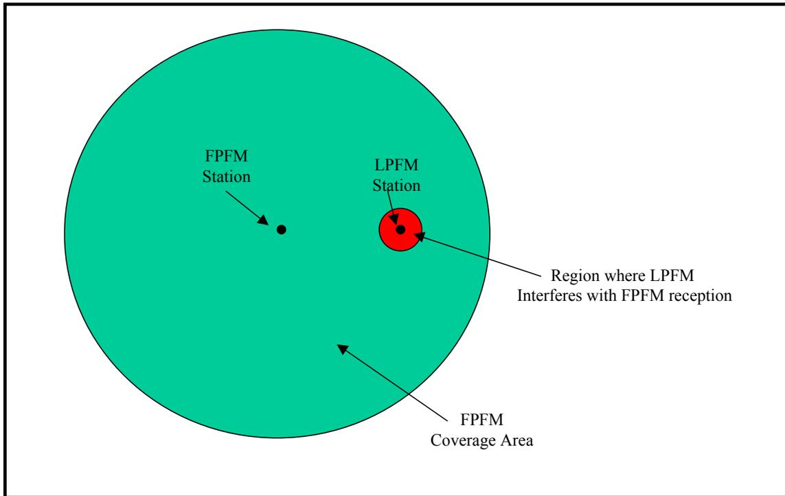
**Figure 4-3. Notional Interference Area**
