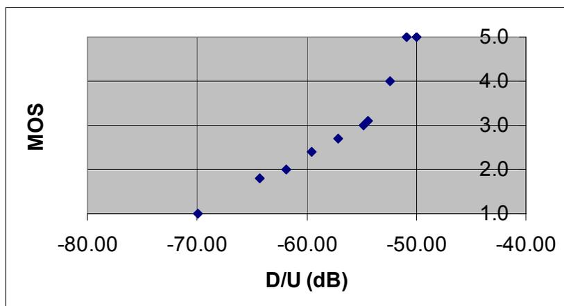
**Figure 3-15. MOS-D/U Measurement for T-P at 52.6 dBu FPFM (FPFM is Victim)**
