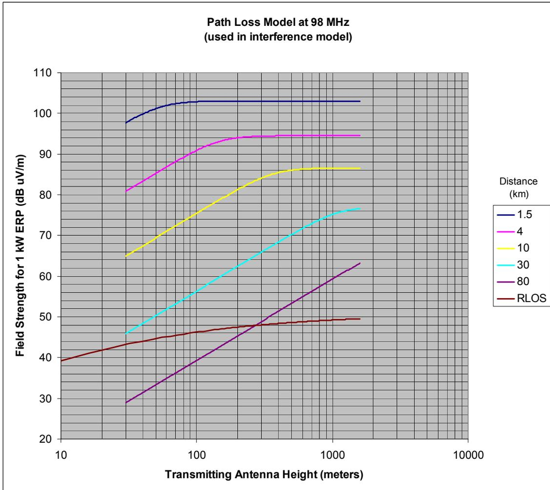
**Figure 4-2. Path Loss Model at 98 MHz**
