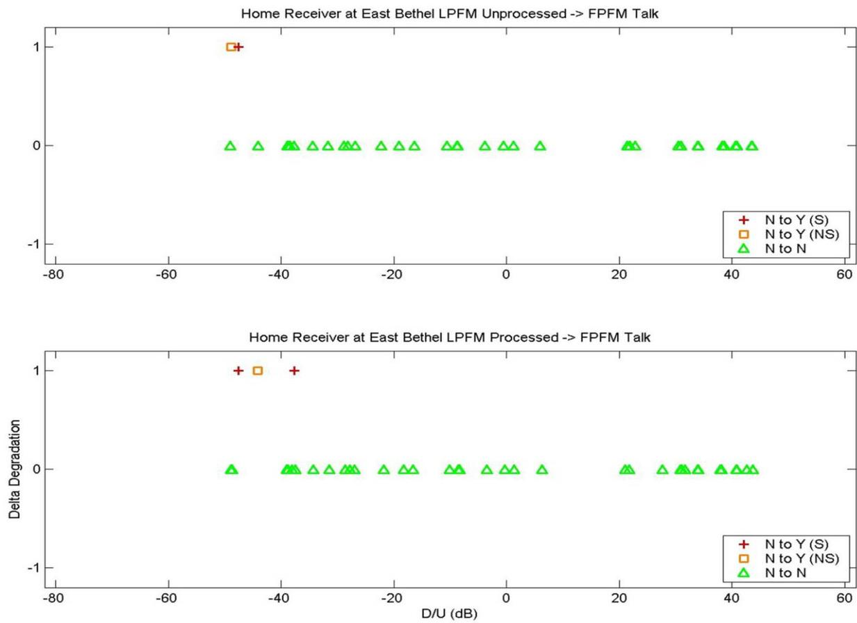
**Figure E-15. Delta Degradation for the Home Receiver at East Bethel and for the Specified LPFM-FPFM Program Content Combinations**
