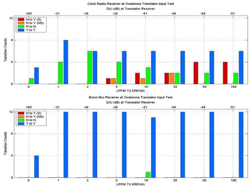
**Figure C-14. Transition Counts for the Clock Radio and Boom Box Receivers at Owatonna Translator Input Test**
