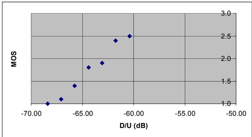
**Figure 3-17. MOS-D/U Measurement for U-T at 52.6 dBu FPFM (FPFM in P, Digital On, SCA is Victim)**
