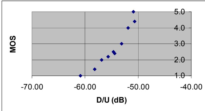
**Figure 3-8. MOS-D/U Measurement for U-T at 58.6 dBu FPFM (FPFM is Victim)**
