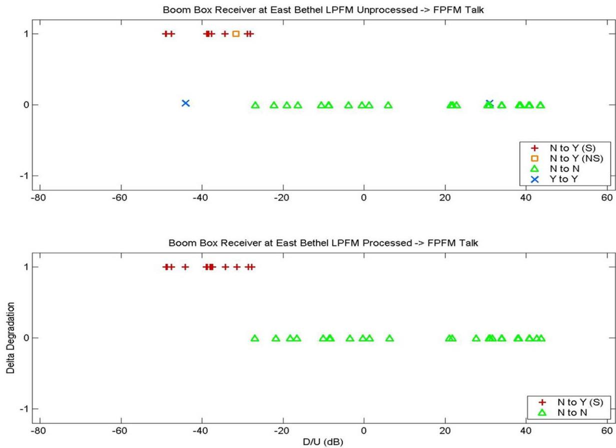
**Figure E-13. Delta Degradation for the Boom Box Receiver at East Bethel and for the Specified LPFM-FPFM Program Content Combinations**
