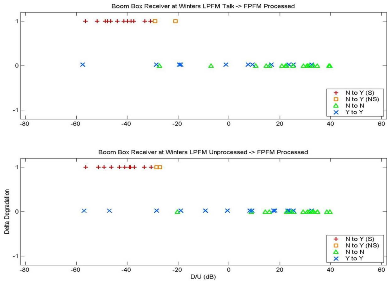
**Figure E-24. Delta Degradation for the Boom Box Receiver at Winters and for the Specified LPFM-FPFM Program Content Combinations**
