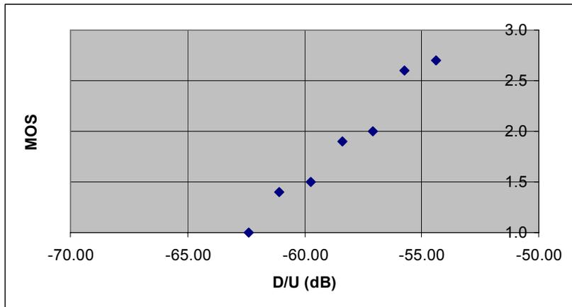
**Figure 3-24. MOS-D/U Measurement for U to T at 58.6 dBu FPFM (FPFM in T, Digital On, SCA is Victim)**
