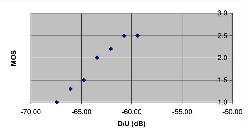
**Figure 3-23. MOS-D/U Measurement for T to T at 52.6 dBu FPFM (FPFM in T, Digital On, SCA is Victim)**
