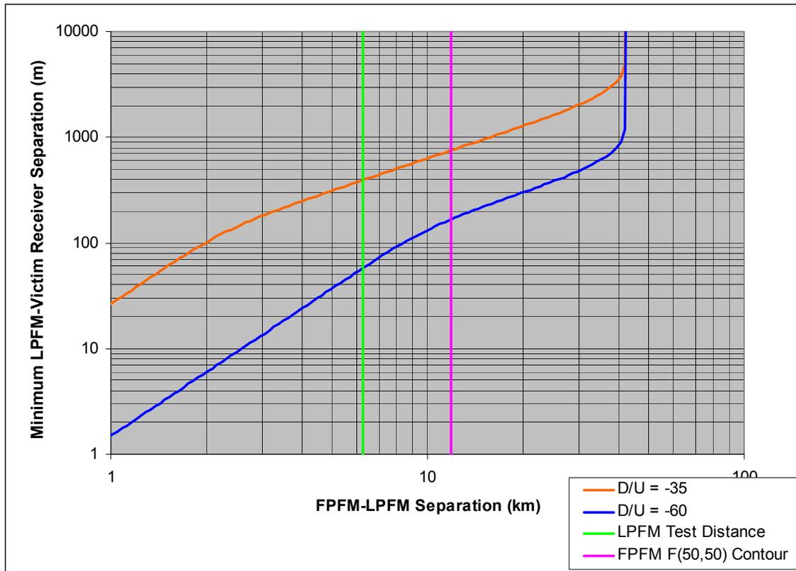
**Figure 4-14. Owatonna Minimum Separation**
