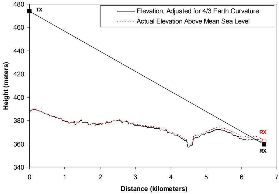
**Figure B-39. Path Profile: K289AE (FPFM) to Owatonna Location 4**
