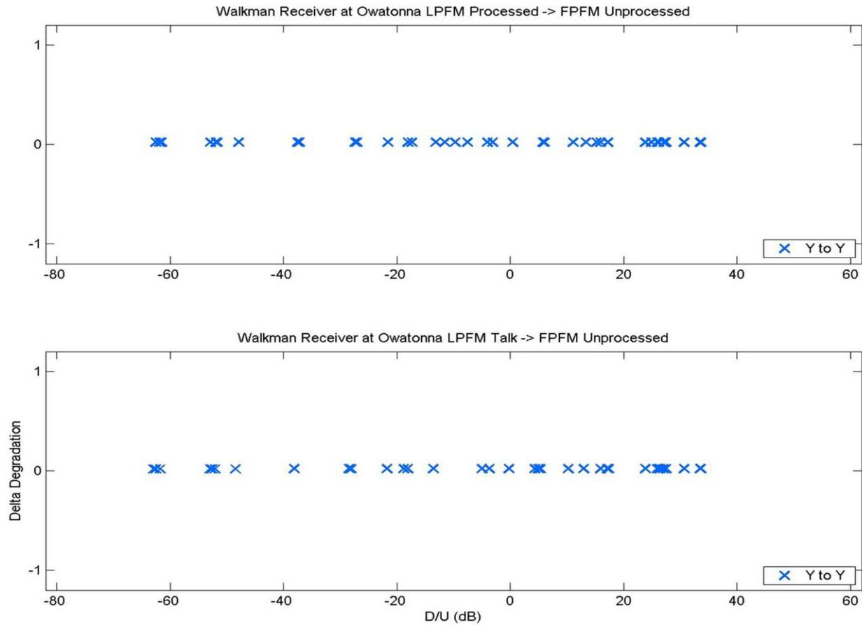
**Figure E-20. Delta Degradation for the Walkman Receiver at Owatonna Translator Output Test and for the Specified LPFM-FPFM Program Content Combinations**
