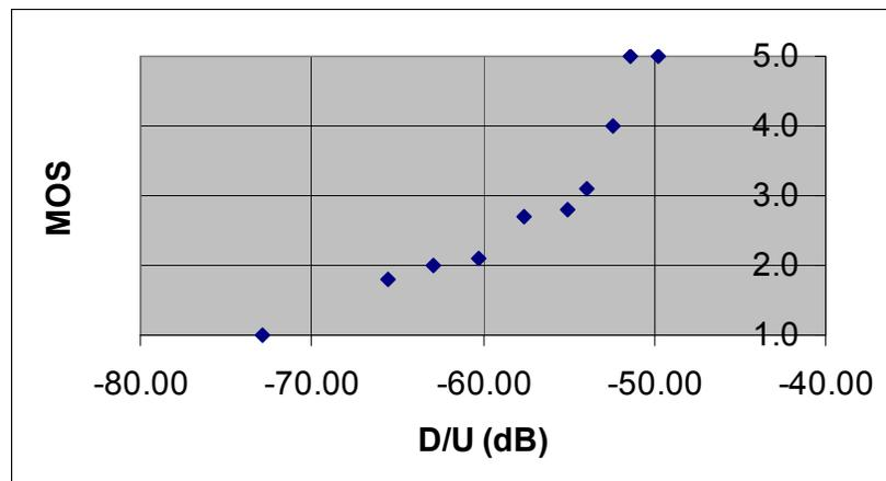
**Figure 3-7. MOS-D/U Measurement for U-U at 52.6 dBu FPFM (FPFM is Victim)**
