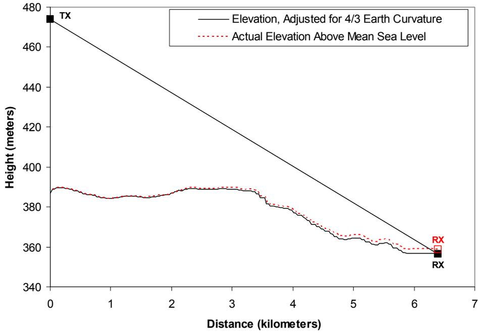
**Figure B-49. Path Profile: K289AE (FPFM) to Owatonna Location 1 (Translator Input)**
