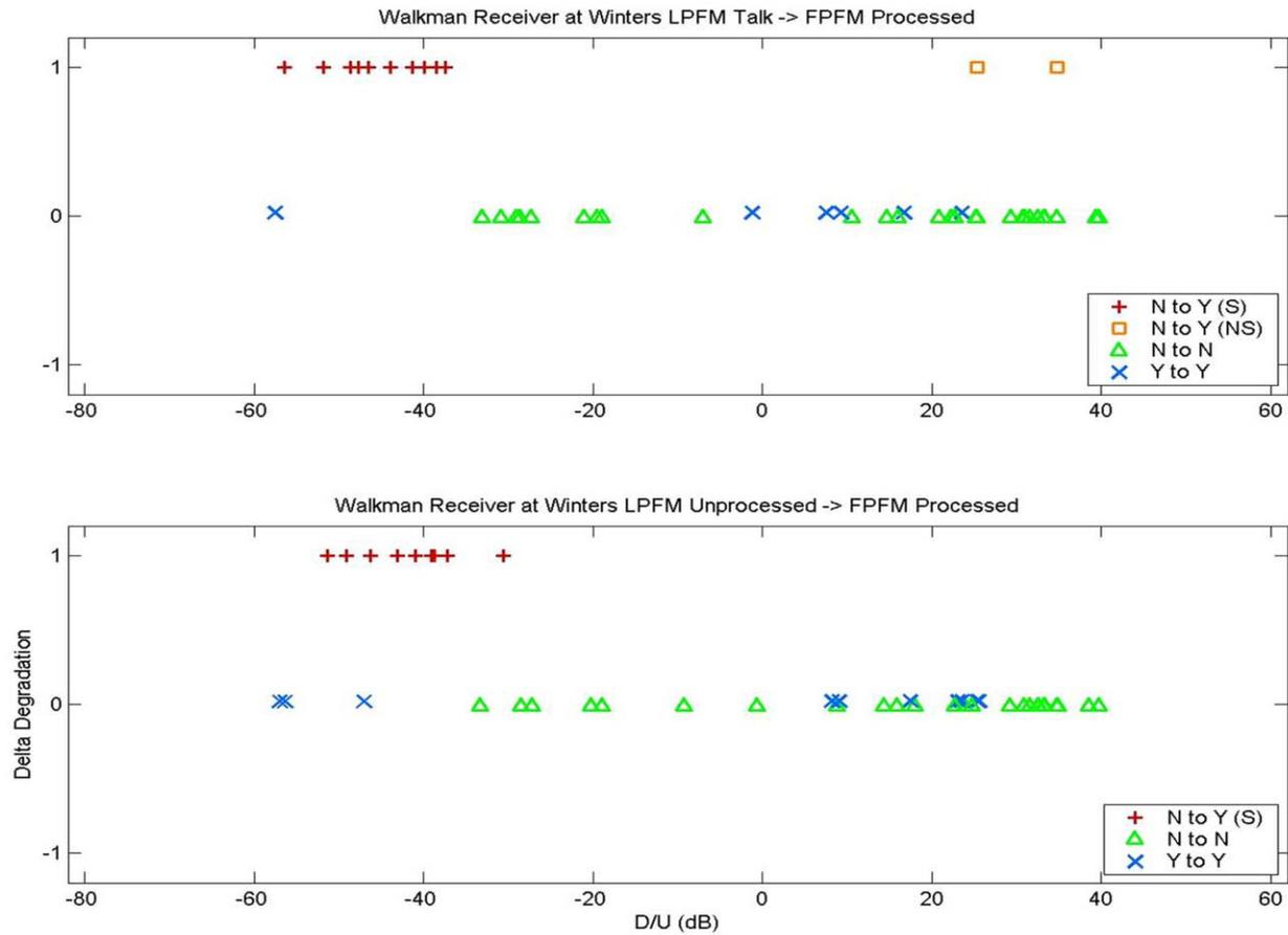
**Figure E-25. Delta Degradation for the Walkman Receiver at Winters and for the Specified LPFM-FPFM Program Content Combinations**
