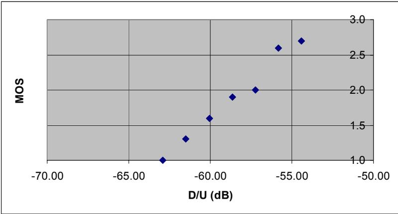
**Figure 3-22. MOS-D/U Measurement for T to T at 58.6 dBu FPFM (FPFM in T, Digital On, SCA is Victim)**
