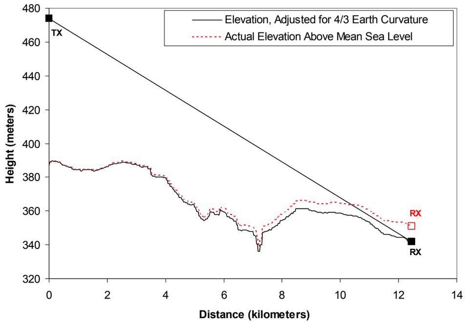
**Figure B-50. Path Profile: K289AE (FPFM) to Owatonna Location 2 (Translator Input)**
