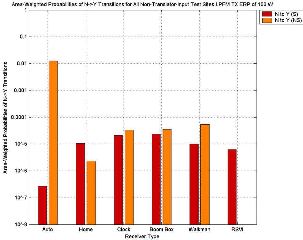
**Figure 2-3. Area-Weighted Probabilities of N→Y Transitions for All Non-Translator-Input Test Sites, LPFM ERP Value of 100 W**
