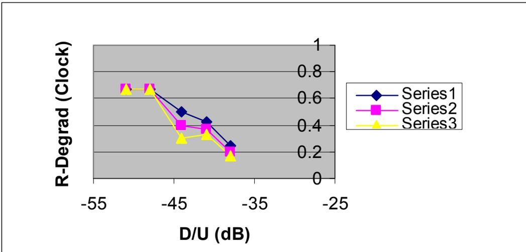
Figure 2-21. Relative Degradation for Clock Radio in FM Translator Test
