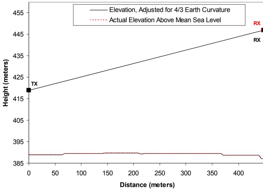
**Figure B-52. Path Profile: Owatonna LPFM (Translator Input) to K289AE (Owatonna Translator)**
