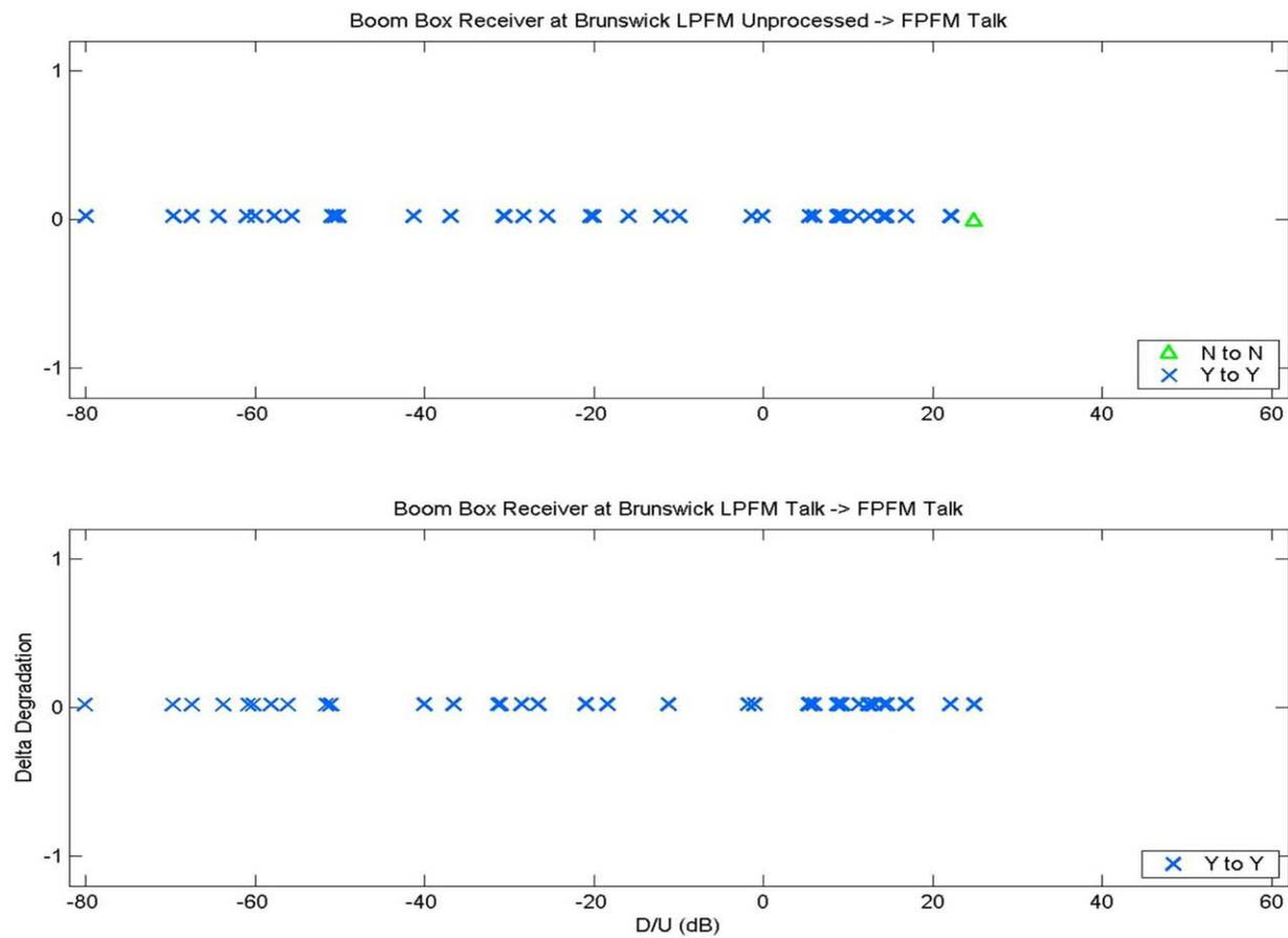
**Figure E-8. Delta Degradation for the Boom Box Receiver at Brunswick and for the Specified LPFM-FPFM Program Content Combinations**
