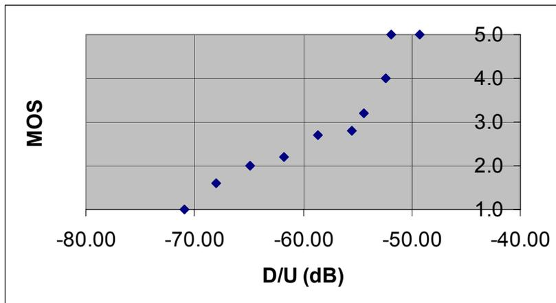
**Figure 3-5. MOS-D/U Measurement for U□P at 52.6 dBu FPFM (FPFM is Victim)**
