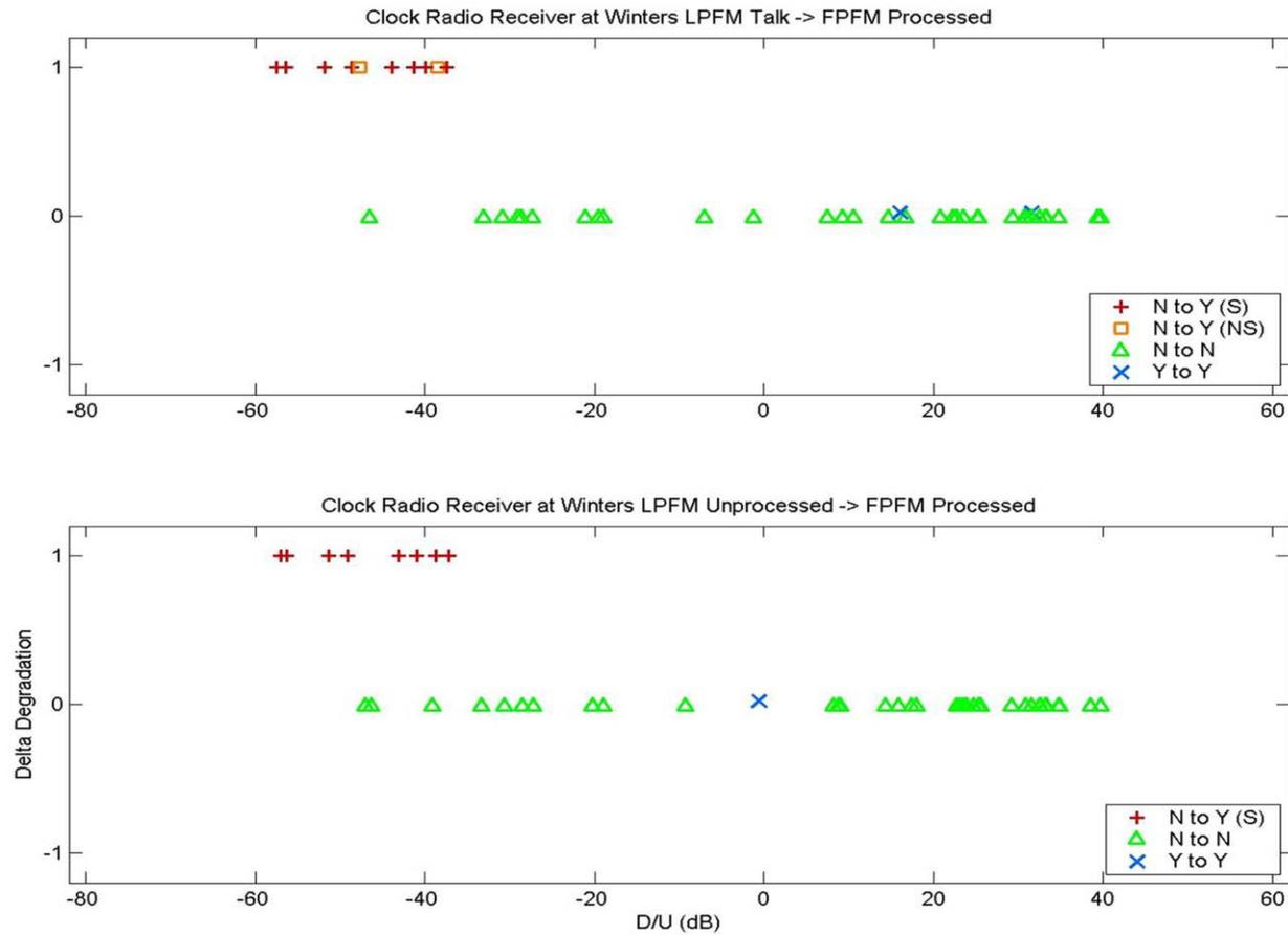
**Figure E-23. Delta Degradation for the Clock Radio Receiver at Winters and for the Specified LPFM-FPFM Program Content Combinations**
