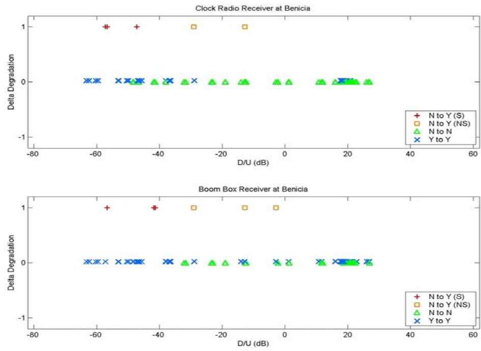
Figure C-20. Delta Degradation for the Clock Radio and Boom Box Receivers at Benicia
