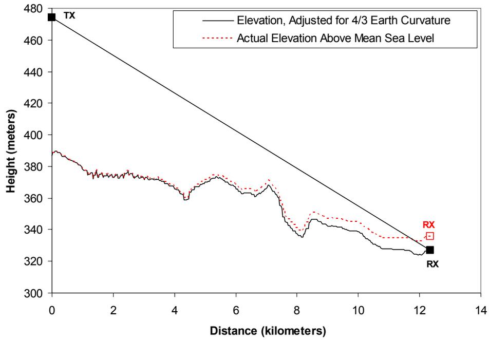
Figure B-45. Path Profile: K289AE (FPFM) to Owatonna Location 7
