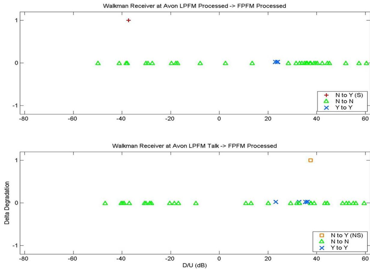
**Figure E-4. Delta Degradation for the Walkman Receiver at Avon and for the Specified LPFM-FPFM Program Content Combinations**
