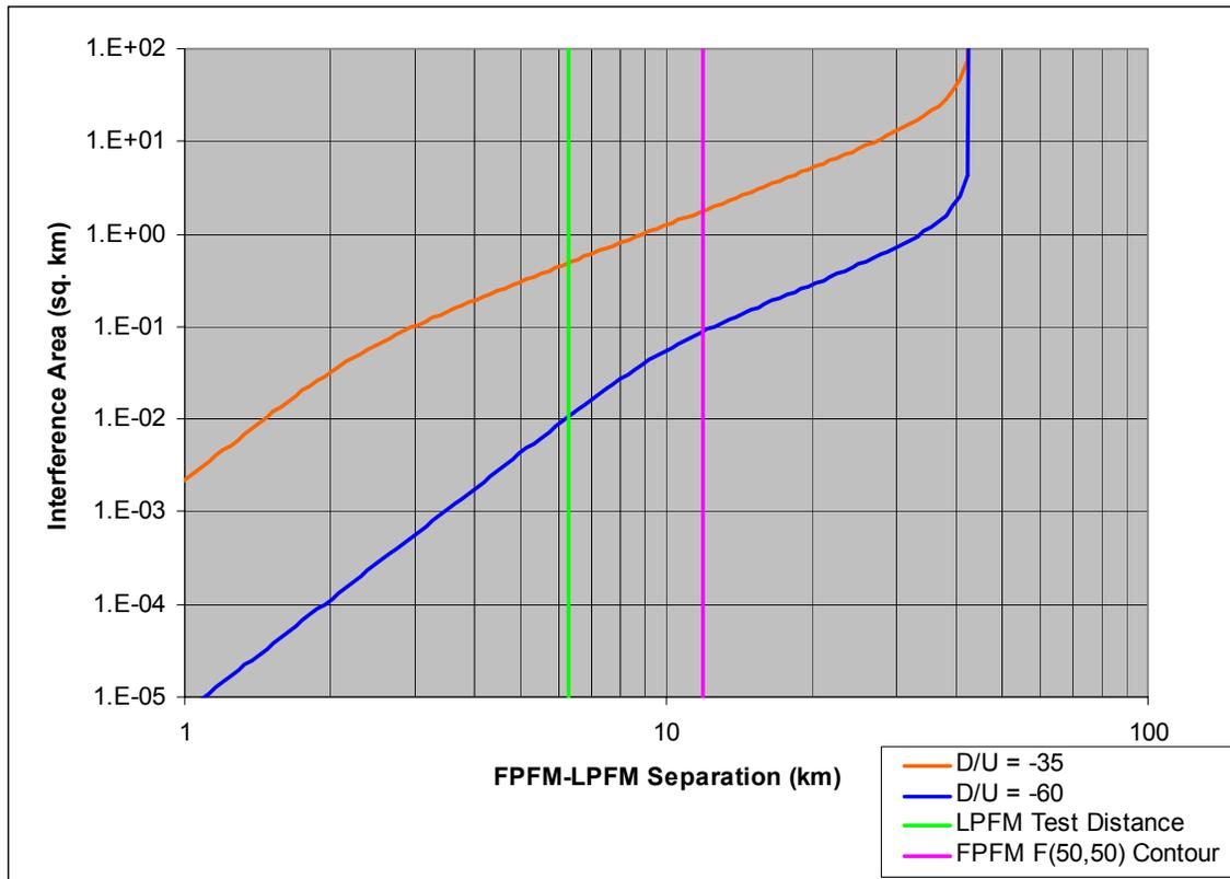
**Figure 4-15. Owatonna Interference Area**
