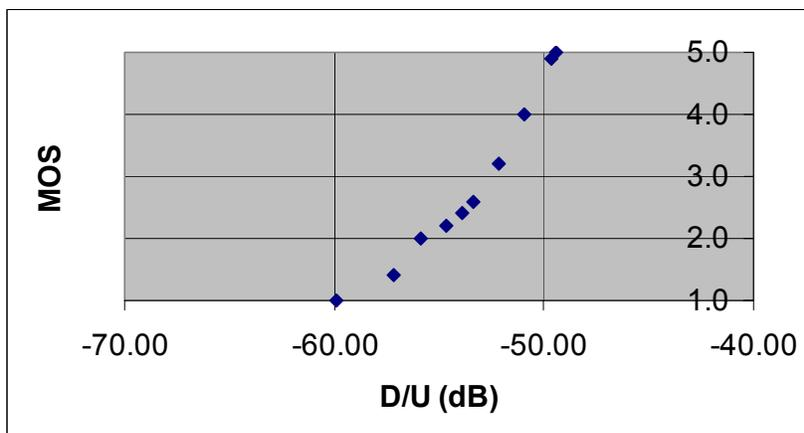
**Figure 3-11. MOS-D/U Measurement for T-T at 52.6 dBu FPFM (FPFM is Victim)**
