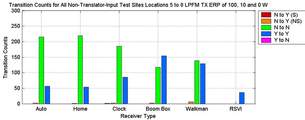
**Figure C-26. Transition Counts for All Non-Translator-Input Test Sites, All LPFM ERP Values (100, 10, and 0 W) and Separating Locations 1 to 4, and Locations 5 to 8 in Two Subplots**
