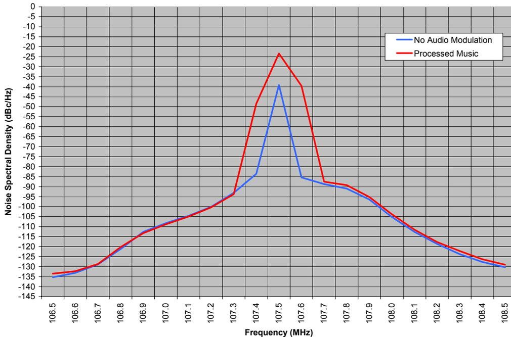
**Figure 2-2. Measured Phase-Noise Spectral Density of LPMF Transmitter**
