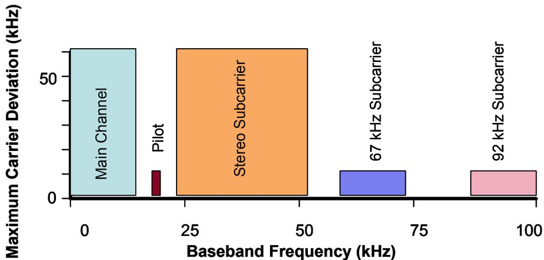
**Figure 2-1. Baseband Structure of an FM Broadcasting Station**
