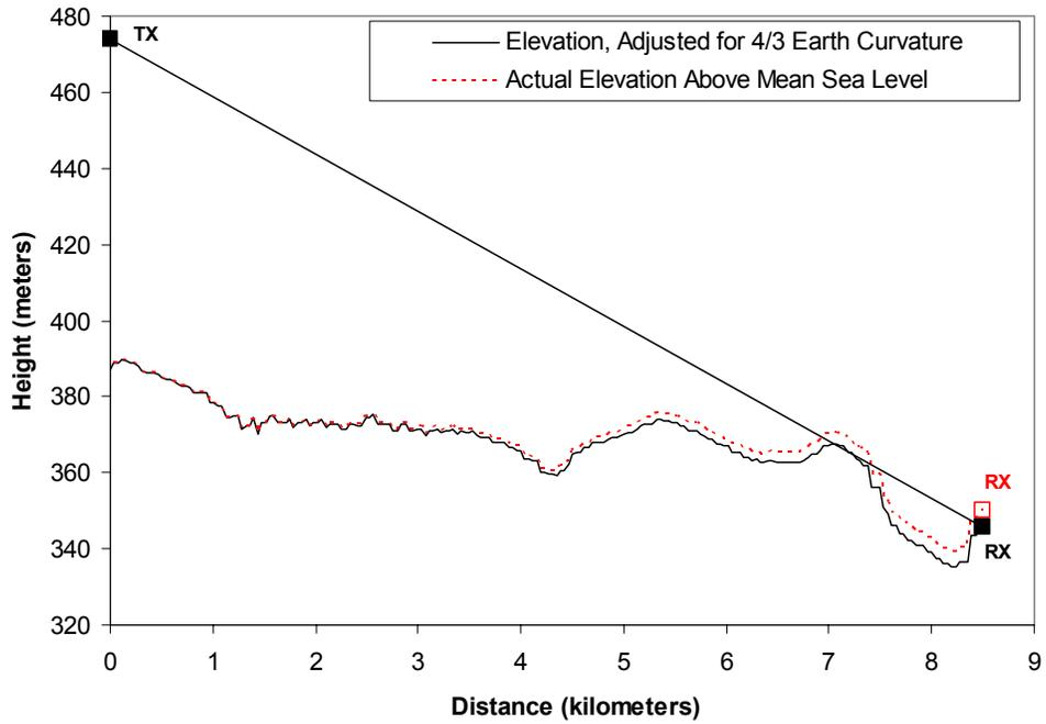
**Figure B-43. Path Profile: K289AE (FPFM) to Owatonna Location 6**
