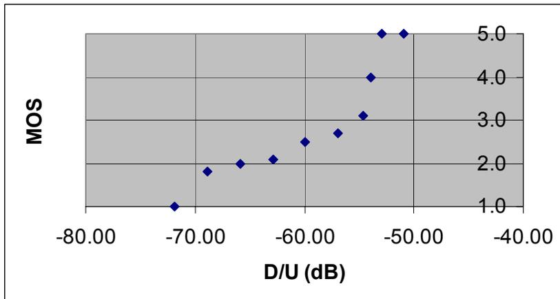
**Figure 3-14. MOS-D/U Measurement for T-P at 58.6 dBu FPFM (FPFM is Victim)**
