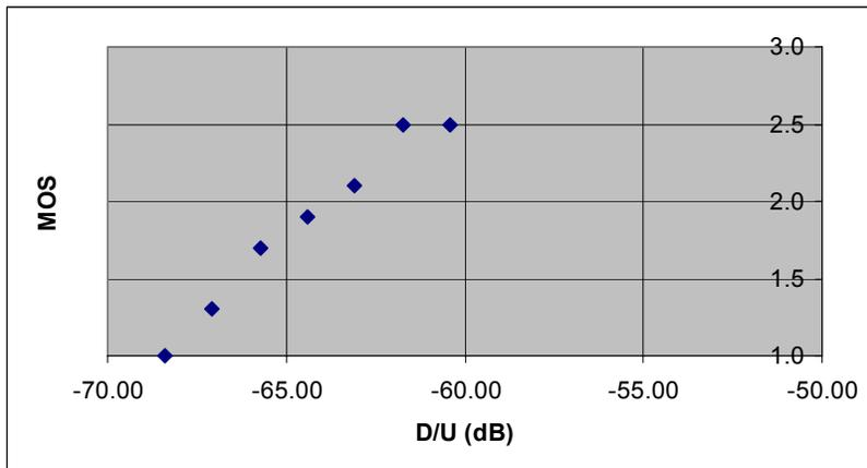
**Figure 3-27. MOS-D/U Measurement for T□T at 52.6 dBu FPFM (FPFM in P, Digital On, SCA is Victim)**
