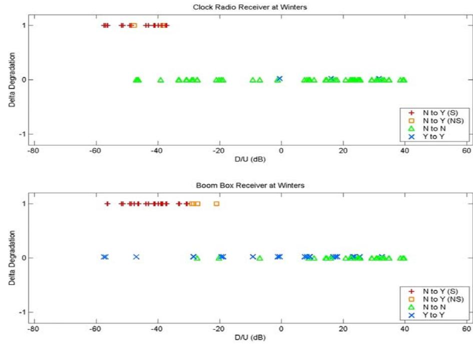
**Figure C-17. Delta Degradation for the Clock Radio and Boom Box Receivers at Winters**
