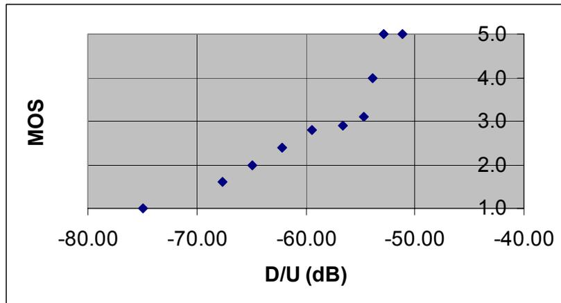
**Figure 3-6. MOS-D/U Measurement for U-U at 58.6 dBu FPFM (FPFM is Victim)**
