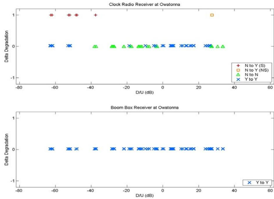
**Figure C-11. Delta Degradation for the Clock Radio and Boom Box Receivers at Owatonna Translator Output Test**
