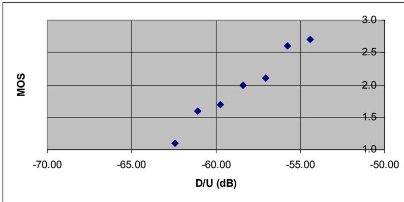
**Figure 3-26. MOS-D/U Measurement for T to T at 58.6 dBu FPFM (FPFM in P, Digital On, SCA is Victim)**
