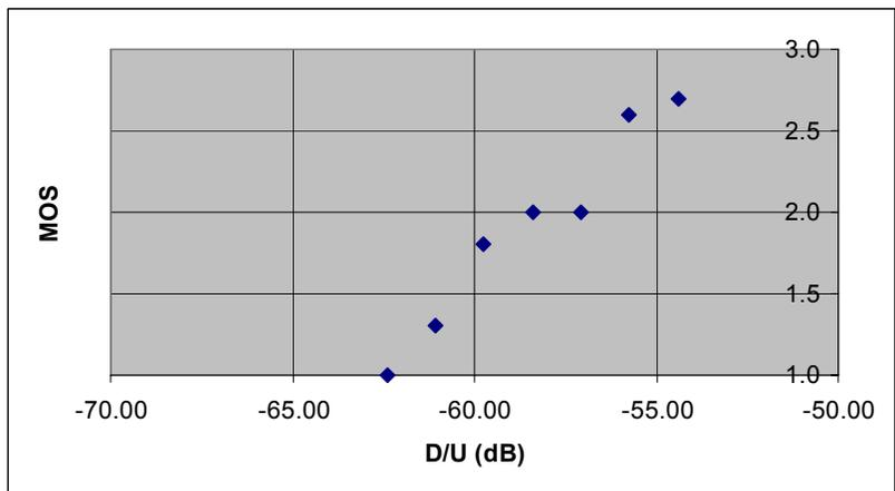
**Figure 3-18. MOS-D/U Measurement for U-T at 58.6 dBu FPFM (FPFM in U, Digital On, SCA is Victim)**
