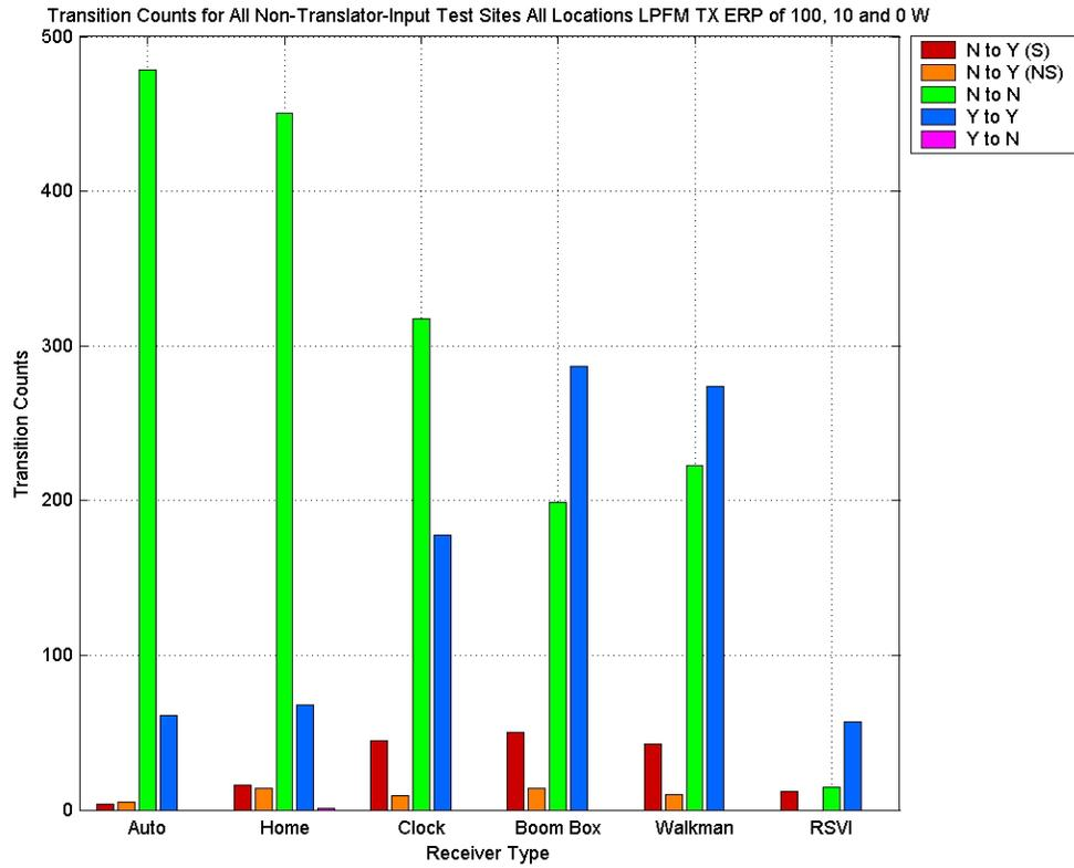
**Figure C-22. Transition Counts for All Non-Translator-Input Test Sites, All Receiver Measurement Locations, All LPFM Values (100, 10, and 0 W)**
