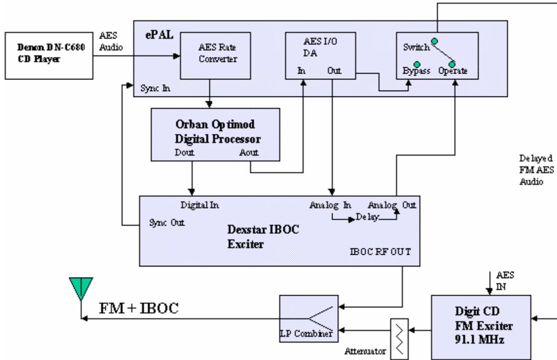
Figure 3-2. Circuit Setup of IBOC Exciter
