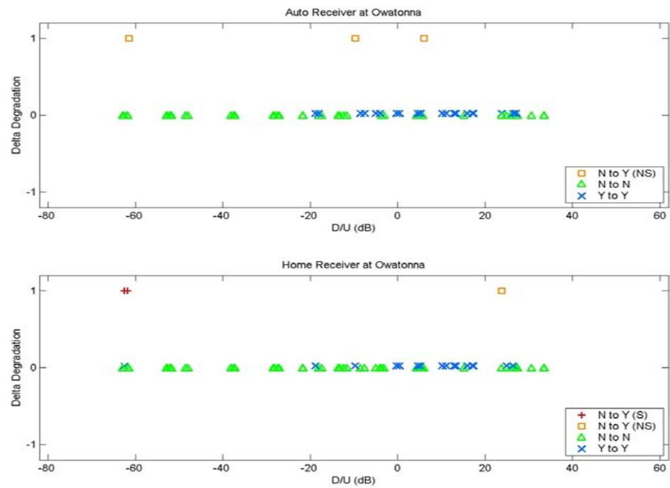
**Figure C-10. Delta Degradation for the Auto and Home Receivers at Owatonna Translator Output Test**
