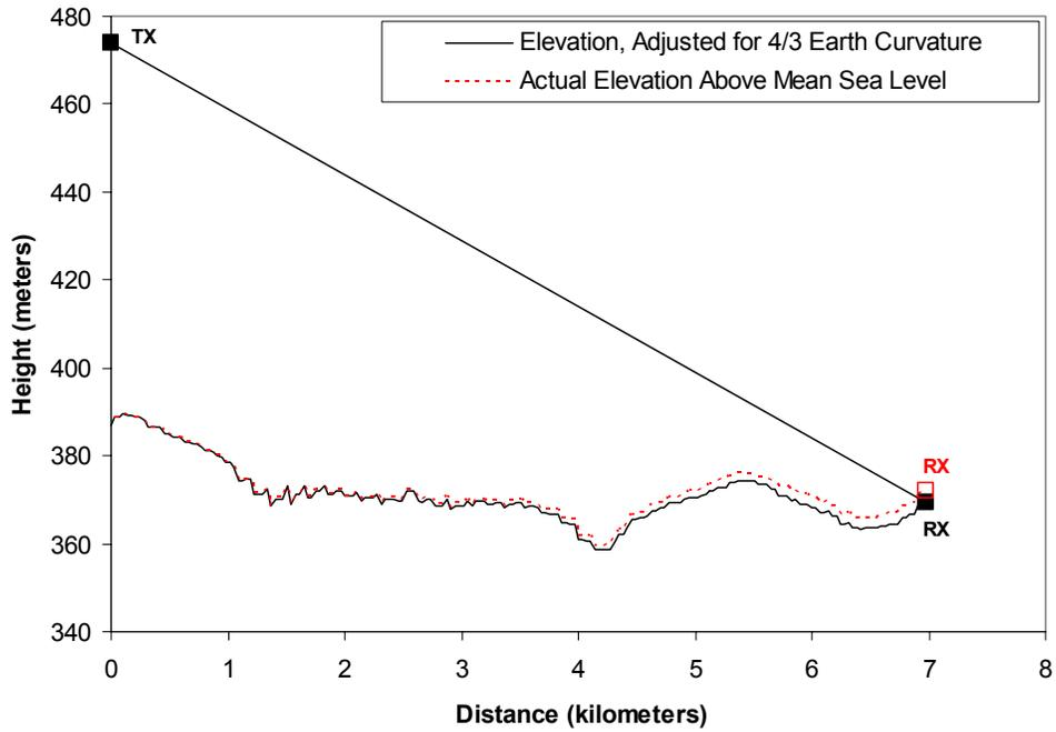
**Figure B-41. Path Profile: K289AE (FPFM) to Owatonna Location 5**
