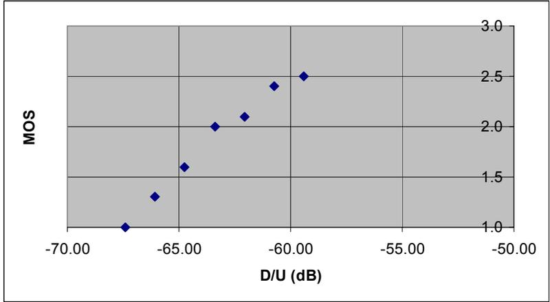
**Figure 3-21. MOS-D/U Measurement for T to T at 52.6 dBu FPFM (FPFM in U, Digital On, SCA is Victim)**
