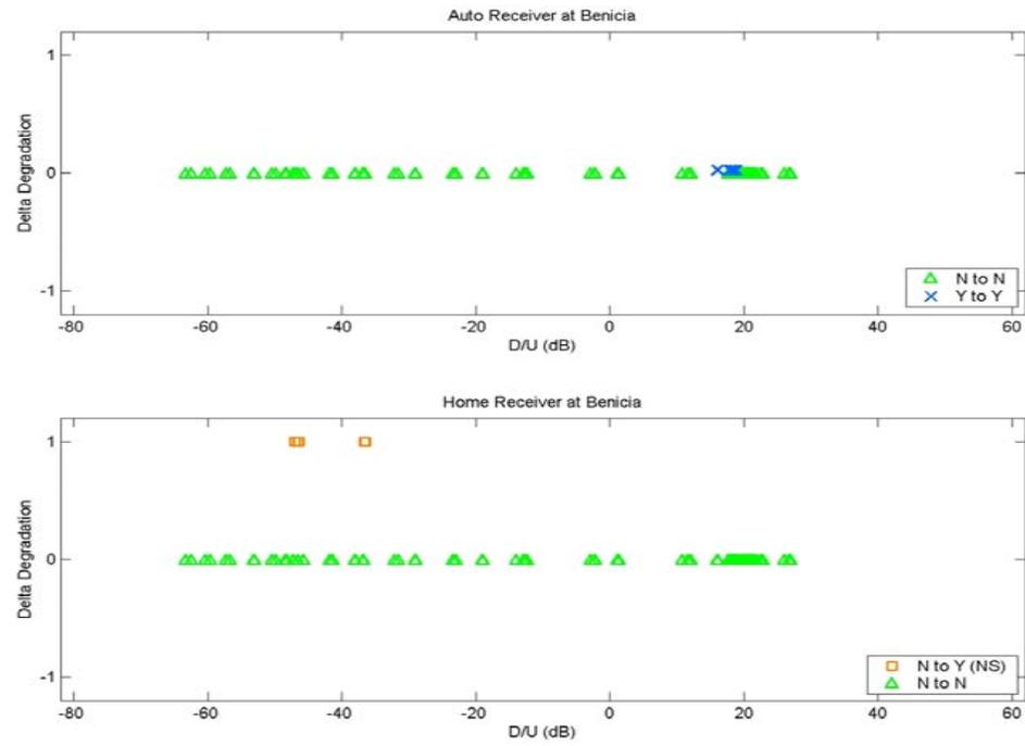
**Figure C-19. Delta Degradation for the Auto and Home Receivers at Benicia**
