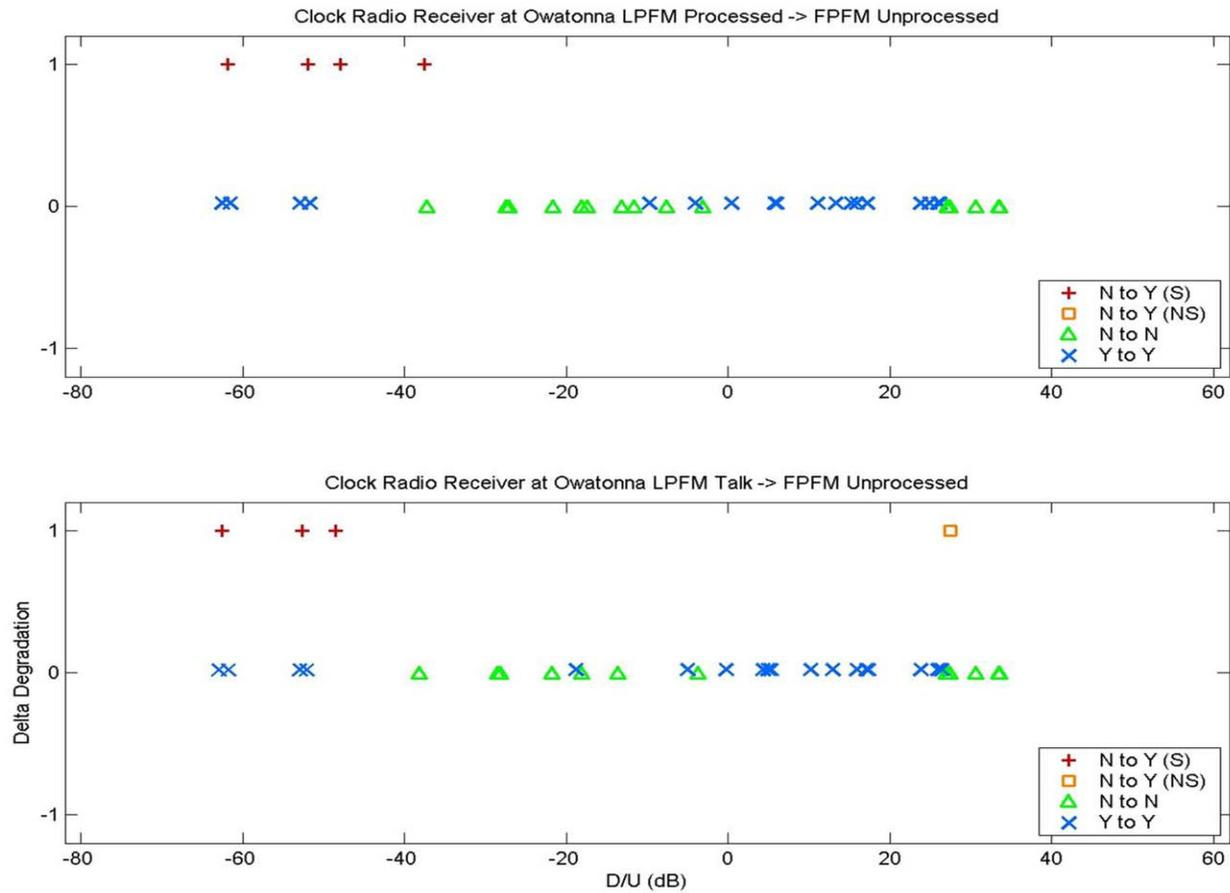
**Figure E-18. Delta Degradation for the Clock Radio Receiver at Owatonna Translator Output Test and for the Specified LPFM-FPFM Program Content Combinations**
