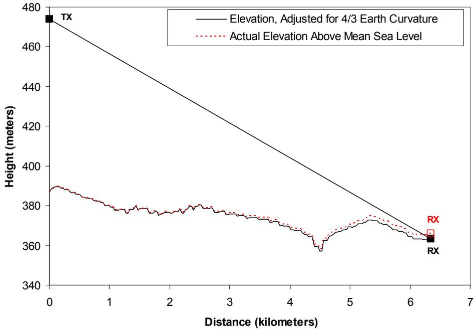
Figure B-37. Path Profile: K289AE (FPFM) to Owatonna Location 3
