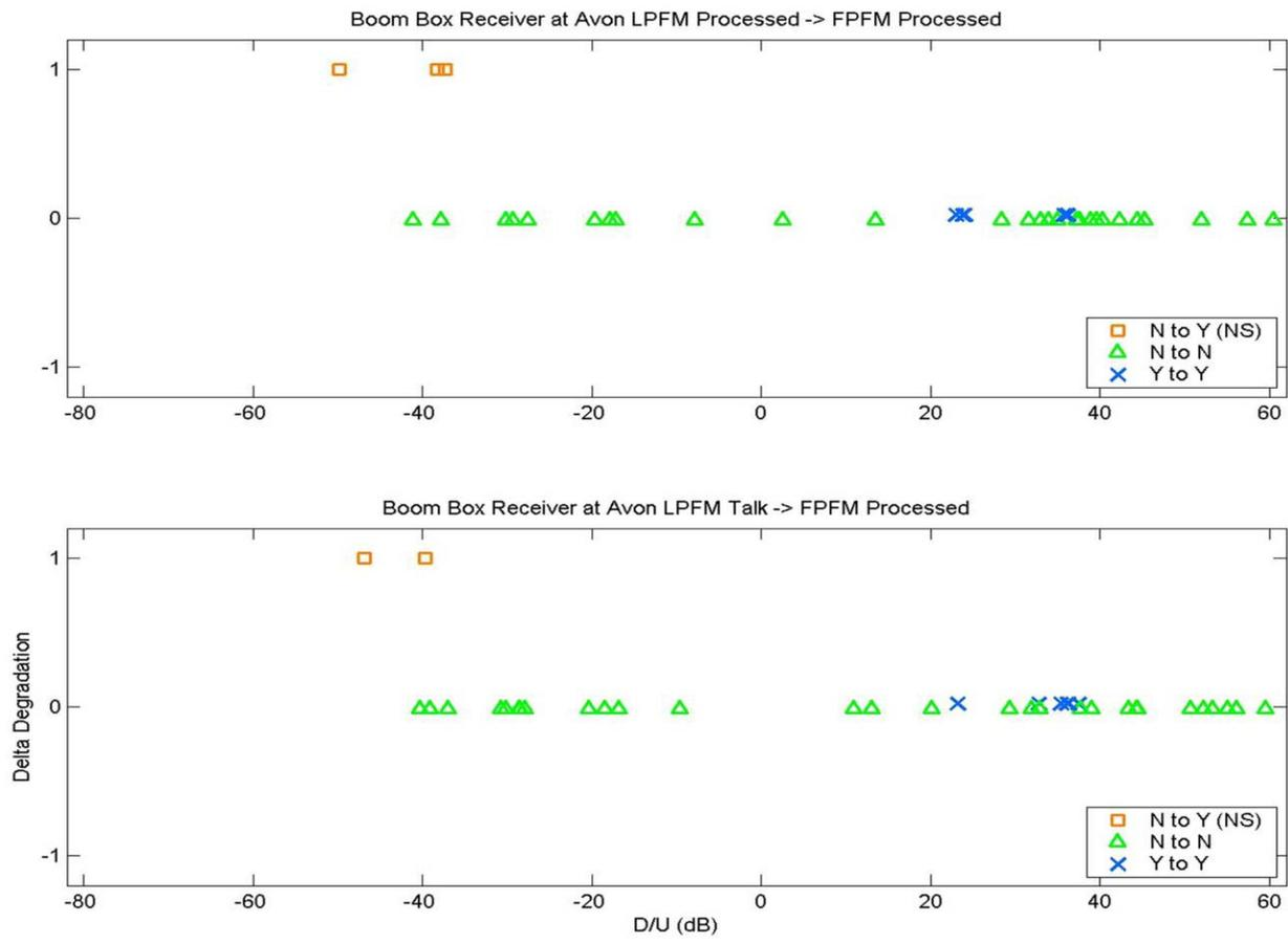
**Figure E-3. Delta Degradation for the Boom Box Receiver at Avon and for the Specified LPFM-FPFM Program Content Combinations**
