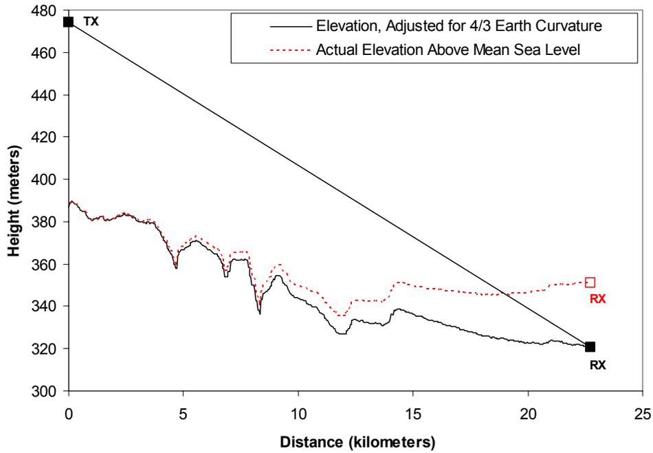
**Figure B-47. Path Profile: K289AE (FPFM) to Owatonna Location 8**
