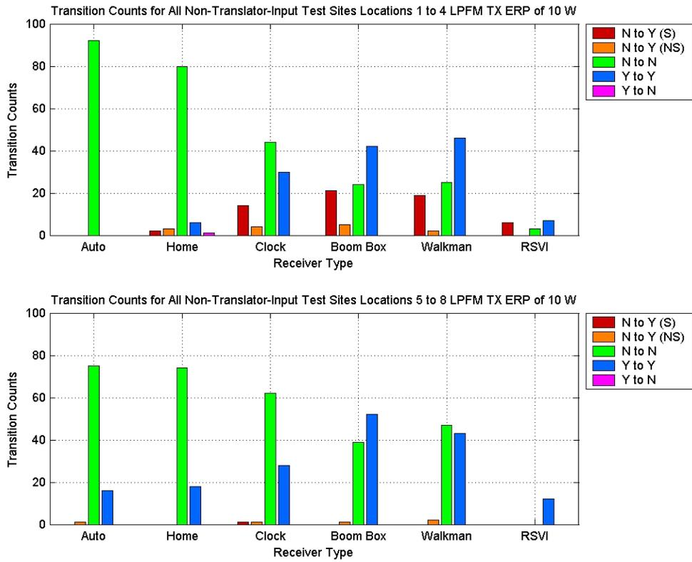
**Figure C-28. Transition Counts for All Non-Translator-Input Test Sites, LPFM ERP Value of 10 W and Separating Locations 1 to 4, and Locations 5 to 8 in Two Subplots**
