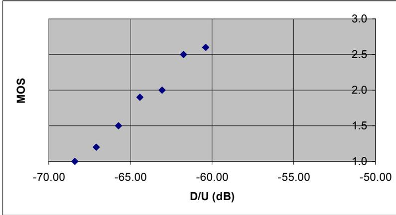
**Figure 3-25. MOS-D/U Measurement for U to T at 52.6 dBu FPFM (FPFM in T, Digital On, SCA is Victim)**
