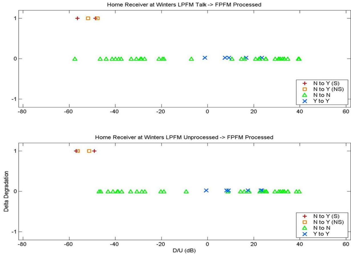
**Figure E-26. Delta Degradation for the Home Receiver at Winters and for the Specified LPFM-FPFM Program Content Combinations**
