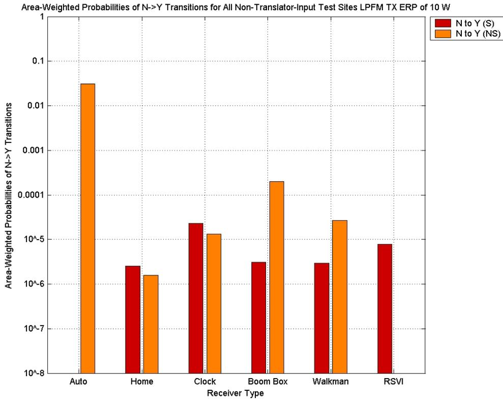
**Figure 2-4. Area-Weighted Probabilities of N→Y Transitions for All Non-Translator-Input Test Sites, LPFM ERP Value of 10 W**
