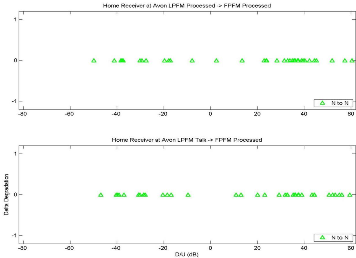
**Figure E-5. Delta Degradation for the Home Receiver at Avon and for the Specified LPFM-FPFM Program Content Combinations**
