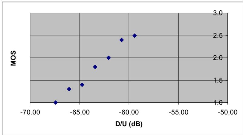
**Figure 3-19. MOS-D/U Measurement for U to T at 52.6 dBu FPFM (FPFM in U, Digital On, SCA is Victim)**
