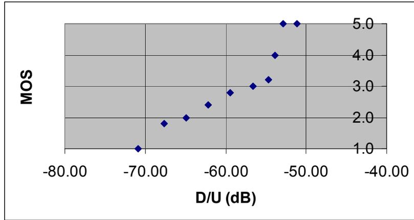
**Figure 3-4. MOS-D/U Measurement for U□P at 58.6 dBu FPFM (FPFM is Victim)**
