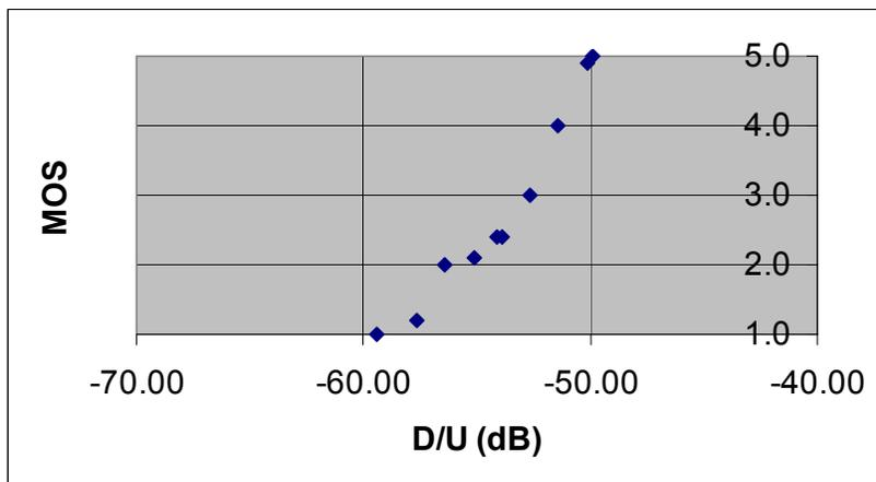
**Figure 3-9. MOS-D/U Measurement for U-T at 52.6 dBu FPFM (FPFM is Victim)**
