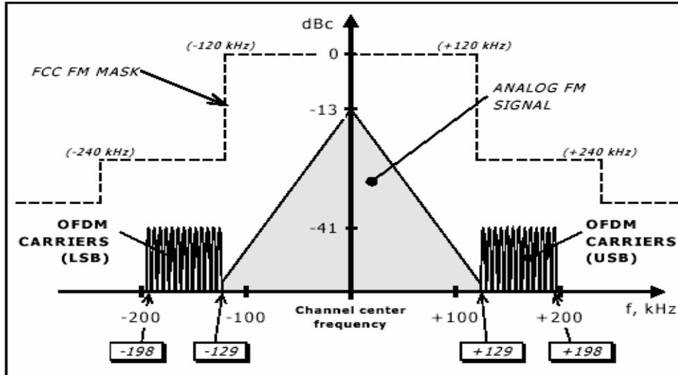
**Figure 3-1. Illustration of FM IBOC Hybrid Mode Spectrum<sup>3</sup>**
