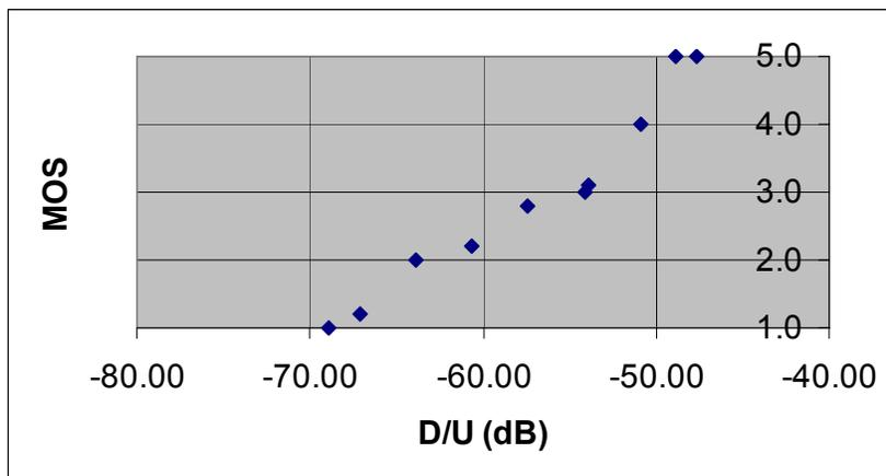
**Figure 3-13. MOS-D/U Measurement for T□U at 52.6 dBu FPFM (FPFM is Victim)**
