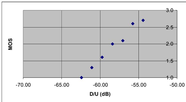
**Figure 3-16. MOS-D/U Measurement for U→T at 58.6 dBu FPFM (FPFM in P, Digital On, SCA is Victim)**
