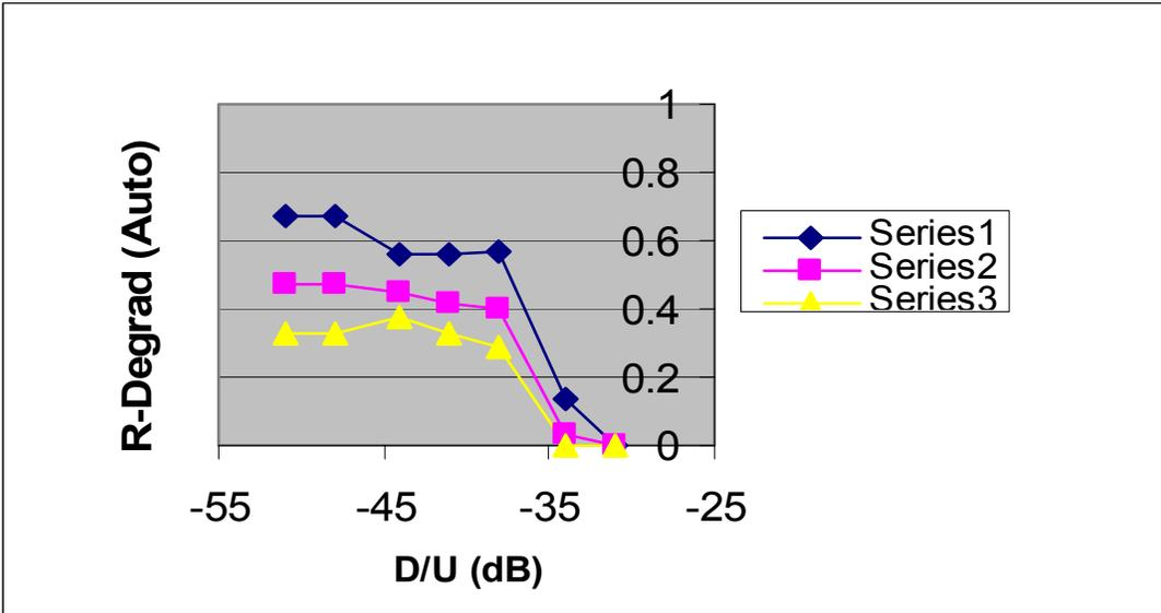
Figure 2-20. Relative Degradation for Auto Radio in FM Translator Test
