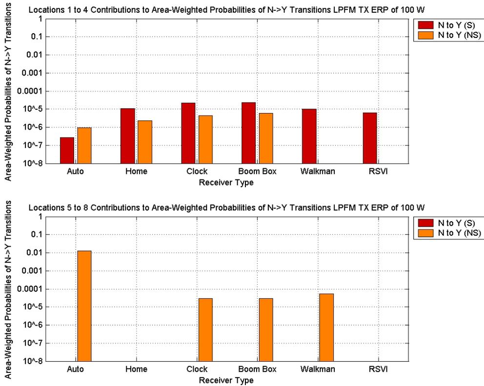
**Figure 2-6. Location Contributions to Area-Weighted Probabilities of N→Y Transitions for All Non-Translator-Input Test Sites, LPFM ERP Value of 100 W**
