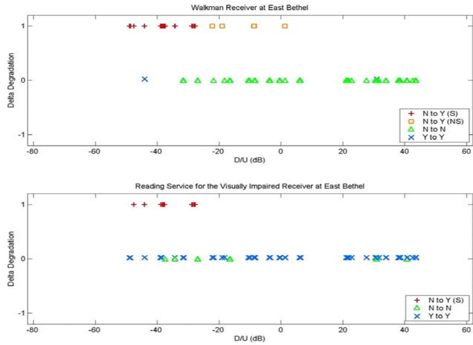
**Figure C-9. Delta Degradation for the Walkman and the RSVI Receivers at East Bethel**
