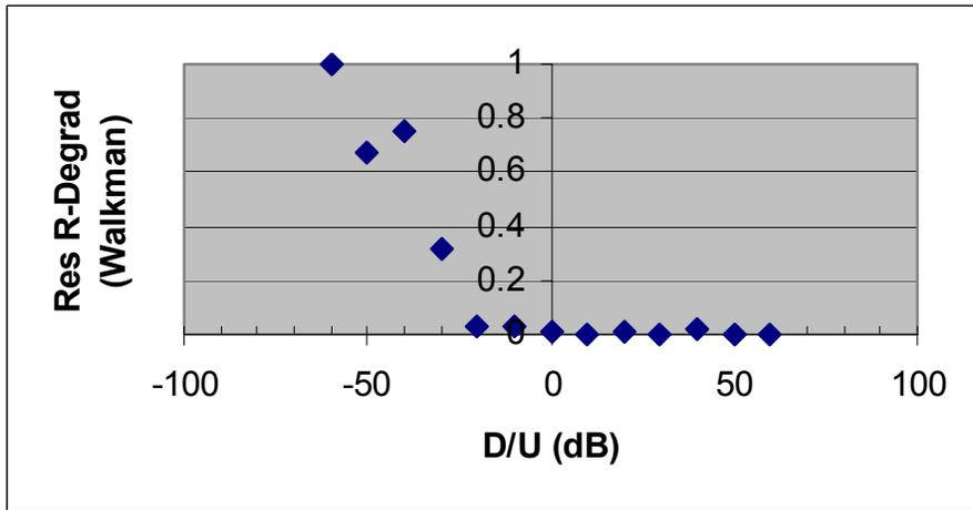
Figure 2-18. Resultant Relative Degradation for Walkman Radio (Case 2)
