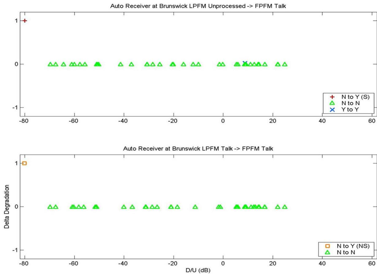
**Figure E-6. Delta Degradation for the Auto Receiver at Brunswick and for the Specified LPFM-FPFM Program Content Combinations**
