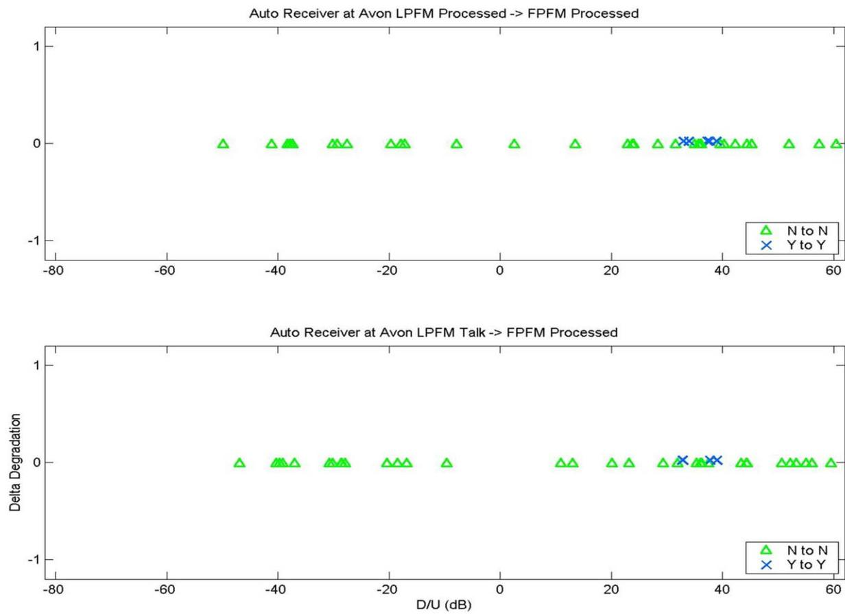
**Figure E-1. Delta Degradation for the Auto Receiver at Avon and for the Specified LPFM-FPFM Program Content Combinations**
