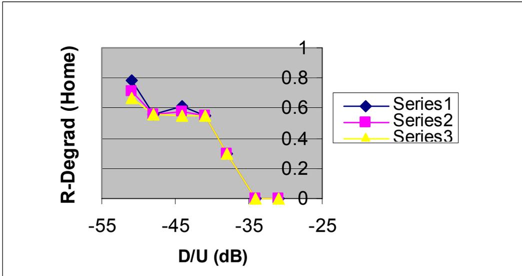
**Figure 2-22. Relative Degradation for Home Radio in FM Translator Test**
