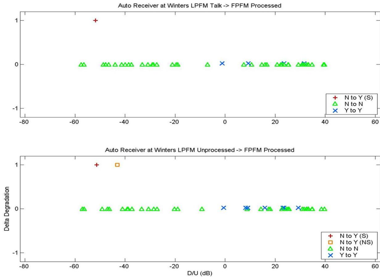
**Figure E-22. Delta Degradation for the Auto Receiver at Winters and for the Specified LPFM-FPFM Program Content Combinations**
