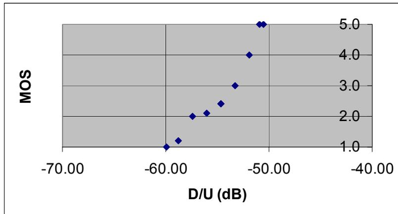
**Figure 3-10. MOS-D/U Measurement for T-T at 58.6 dBu FPFM (FPFM is Victim)**
