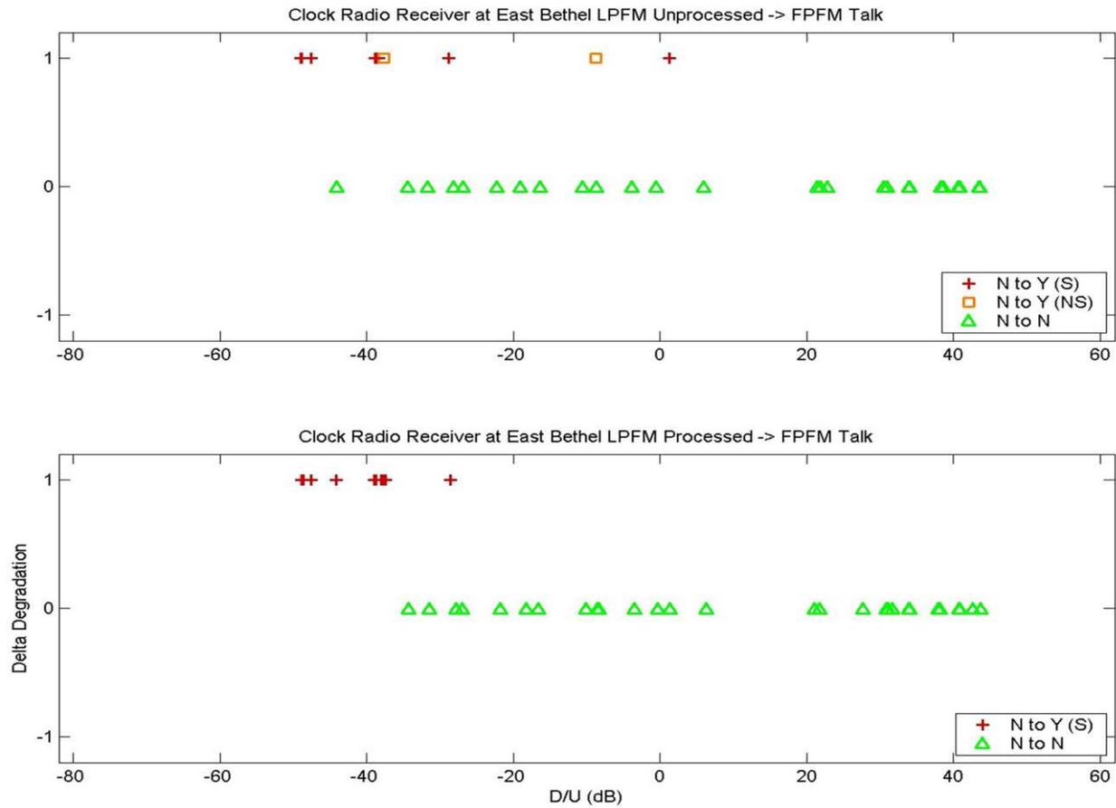
**Figure E-12. Delta Degradation for the Clock Radio Receiver at East Bethel and for the Specified LPFM-FPFM Program Content Combinations**
