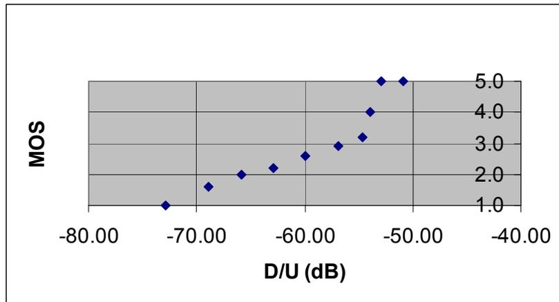
**Figure 3-12. MOS-D/U Measurement for T□U at 58.6 dBu FPFM (FPFM is Victim)**
