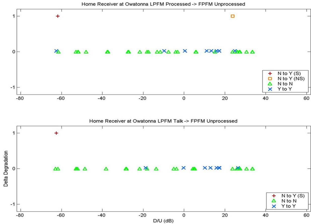
**Figure E-21. Delta Degradation for the Home Receiver at Owatonna Translator Output Test and for the Specified LPFM-FPFM Program Content Combinations**
