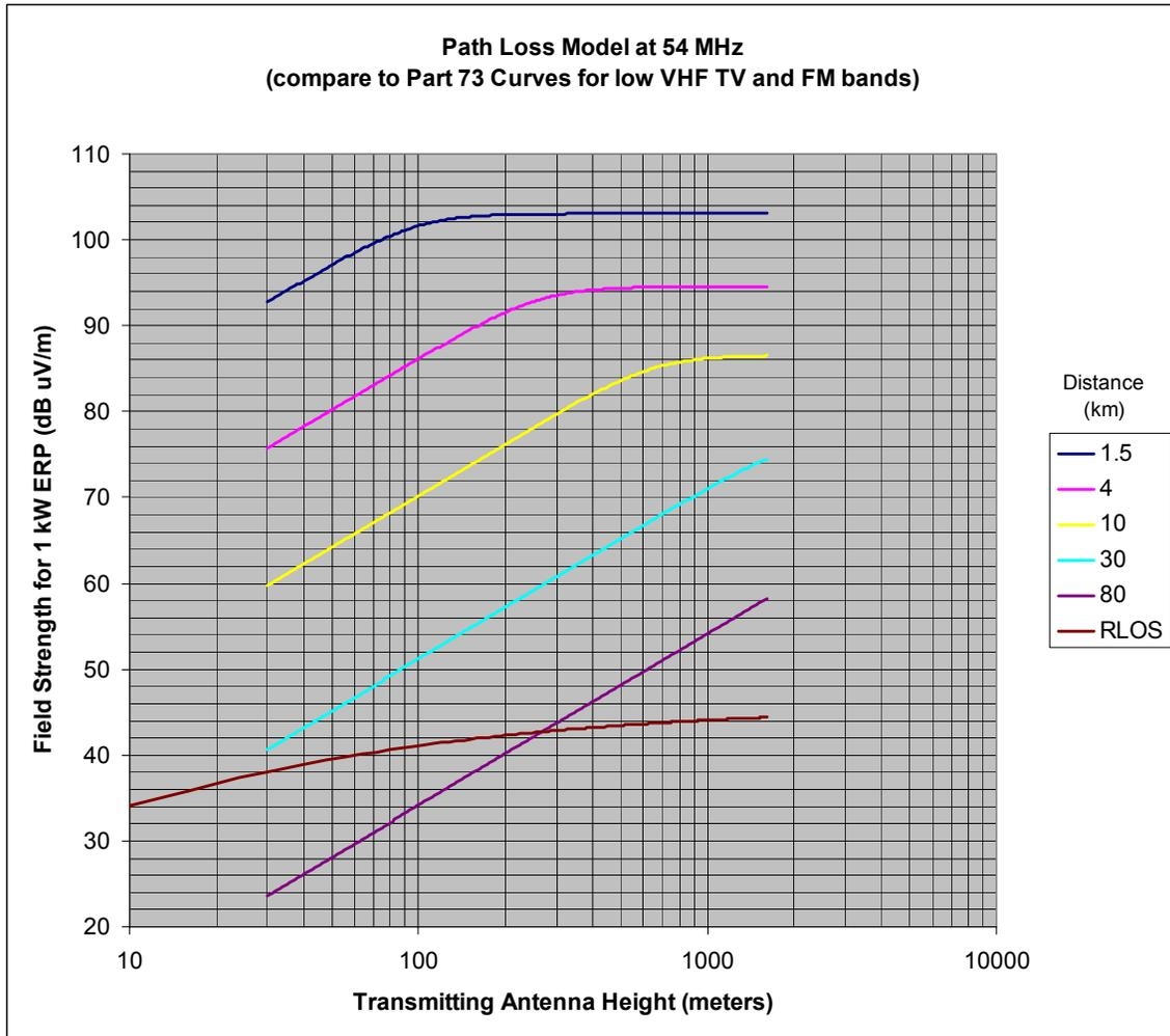
**Figure 4-1. Path Loss Model at 54 MHz (for Comparison to Part 73 Curves)**
