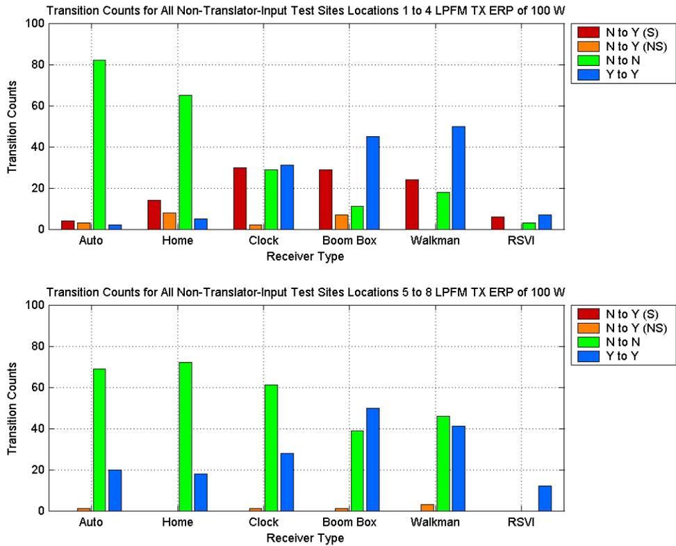
**Figure C-27. Transition Counts for All Non-Translator-Input Test Sites, LPFM ERP Value of 100 W and Separating Locations 1 to 4, and Locations 5 to 8 in Two Subplots**
