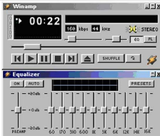
Equalizers improve sound quality by changing the volume of audio at specific frequencies. For example, if an audio signal contains too much bass, compensation can be made by reducing the lower frequency knobs of the equalizer. One trick to improving the “loudness” of audio is to increase the treble frequencies (the right side of the equalizer). This gives the audio more punch, and makes voices more recognizable. Equalizers are very similar
